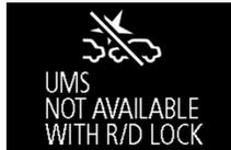
In the following conditions, even if the UMS is ON, the UMS is automatically switched to OFF. In addition, when the UMS is OFF, the UMS is not switched to ON even if the FCM and UMS ON/OFF switch is pressed.
