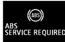
If there is a malfunction in the system, the ABS warning lamp will come on and the warning display will appear on the information screen in the multi information display. Under normal conditions, the ABS warning lamp comes on when the ignition switch is turned to the “ON” position or the operation mode is put in ON and goes off a few seconds later.
