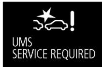
When the warning display appears, the UMS does not operate normally because there are some malfunctions in the system or the sensor. Have the vehicle inspected at an authorised MITSUBISHI MOTORS dealer as soon as possible.
