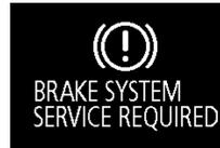
When the ignition switch or the operation mode is put in ON, if the brake fluid is low, this warning is displayed.
