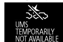
When the warning display appears, the sensors are temporarily not available for some reason such as the environmental condition or increase of the sensor temperature. When the warning display does not disappear after waiting for a while, contact an authorised MITSUBISHI MOTORS dealer.
