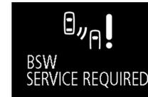
When the warning display appears, the BSW does not operate normally because there are some malfunctions in the system or the sensor. Have the vehicle inspected at an authorised MITSUBISHI MOTORS dealer as soon as possible.
