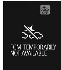
If the system becomes temporarily unavailable due to the high or low temperature of the sensor, the following message will appear.
