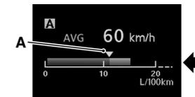
The “A” mark (A) in the momentary fuel gauge shows the average fuel consumption. When the momentary fuel consumption surpasses the average fuel consumption, the
