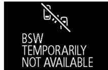
When the warning display appears, the sensor is temporarily not available for some reason such as the environmental condition or increase of the sensor temperature. When the warning display does not disappear after waiting for a while, contact an authorised MITSUBISHI MOTORS dealer.
