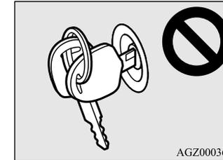
In cases like these, remove the object or additional key from the vehicle key. Then try again to start the engine. If the engine does not start, contact an authorised MITSUBISHI MOTORS dealer.
