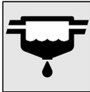
This indicator lamp illuminates when the ignition switch is turned to the “ON” position or the operation mode is put in ON, and goes off after the engine has started. If it lights up while the engine is running, it indicates that water has accumulated inside the fuel filter; if this happens, take action as follows.
