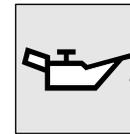
This lamp illuminates when the ignition switch is turned to the "ON" position or the operation mode is put in ON, and the lamp goes off after the engine has started. If it illuminates while the engine is running, the oil pressure is too low. If the warning lamp illuminates while the engine is running, turn the engine off and contact your nearest authorised MITSUBISHI MOTORS dealer for inspection.
