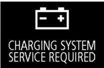
If there is a fault with the charging system, the warning display is displayed on the infor-
