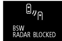
When the warning display appears, the sensor cannot detect a vehicle travelling side by side or an approaching vehicle, because foreign objects, such as dirt, snow or ice, adhere to the bumper surface around the sensor. Remove a dirt, freezing or foreign material on the bumper surface around the sensor. When the warning display does not disappear after having cleaned the sensor, contact an authorised MITSUBISHI MOTORS dealer.
