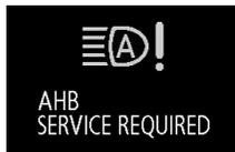
[When the sensor is malfunctioning]
