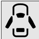
This lamp illuminates when a door is either open or not completely closed.
